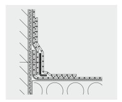
If line fastening with **rigid clamping bars**, the bars must be waterproofed using an unbacked tape.
