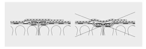
The fasteners must be driven in only so far as to permanently prevent rotation of the load distribution plates and to ensure that the latter press the waterproofing membranes against the substrate without wrinkles.
