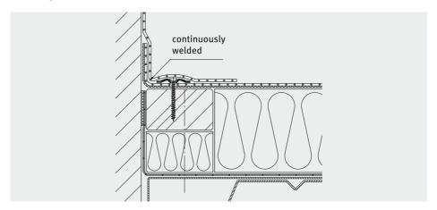
The perimeter fastening of EVALON® waterproofing membranes can be done with approved membrane fasteners (min. 3 fasteners/m) set in a row.
