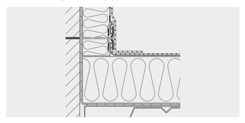
Generally, between the individual fasteners the flashing sheet must also be completely welded in the valley.
