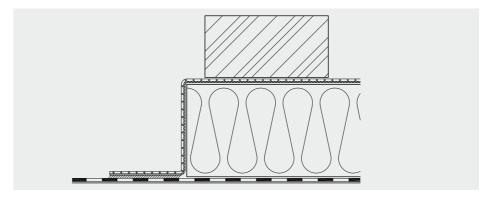
On substrates such as vapour barriers consisting of foils on which bonding is not permissible, the temporary securing of the edge can be done with a folded-back membrane tape and additional ballast.
