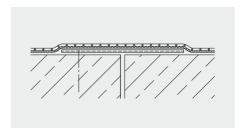
Waterproofing of **type II** joints (DIN 18531): Depending on the extent and the frequency of expansion joints, the type of sealing is to be decided upon individually, e.g.
