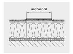
Overlaps of membrane type backings at the joints of thermal insulation layers must not be bonded.
