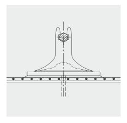
On mechanically fastened waterproofing membranes, the lightning conductor holders are placed directly next to the membrane fasteners.
