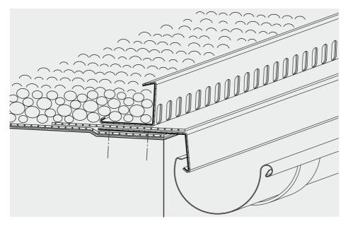
At roof slopes > 3° to  $\leq$  5°, first an unbacked EVALON® tape (approx. 20 cm) is welded over the whole length to the centre of the underneath of the non-perforated, 8 cm wide flange of the gravel stop profile. The edges of this tape are then welded at the required width, along the trough, to the mechanically fastened drip edge made of EVALON® coated metal sheet, and to the roof waterproofing.
