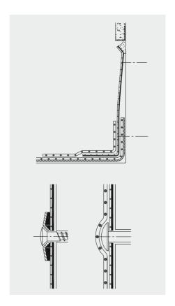
In the area of used roofs, the connection area must be protected against mechanical influences (e.g. with alwitra wall flashing profile WA 1 - ÜK).
