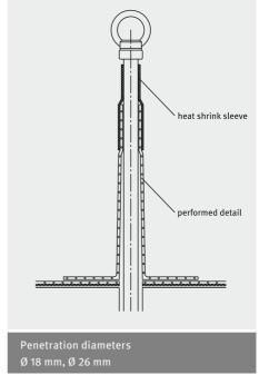
At roof penetrations with a diameter of approx. 8 - 10 mm (e.g. lightning conductor), prior to placing the heat shrink sleeve, the spacer (included with the parts for sleeves Ø 18 mm) must be installed between the roof penetration and the preformed detail according to the illustration.
