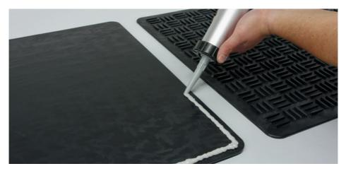
It is recommended to install the tiles with a joint spacing of more than 50 mm. alwitra EVATACK may be visible at some parts along the edges. One cartridge will bond approx. 3 maintenance walkway tiles.
