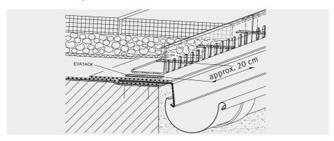
When installing, allow for sufficient joint width (cf. table). At the joint area, butt connectors must be applied.
