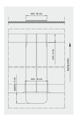
After chamfering, the strip will be seal-welded at its longitudinal edges and at the rounded-off end. Be especially careful when welding the chamfered areas with hot air (hot-air hand tool).
