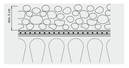
The weight of gravel (16/32 mm) is approx. 18 kg/m² (≈0.18 kN/m²) per 1 cm fill height.
