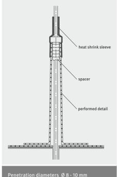
Penetration diameters Ø 8 - 10 mm
