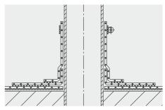
Homogeneously weld the collar at a width of min. 2 cm all around the outer edge to the roof waterproofing, install a stainless steel pipe clamp on the sleeve to make it rainproof.
