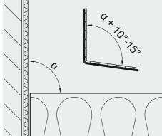
With **coated metal** strips the same effect will be reached by reverse bending.
