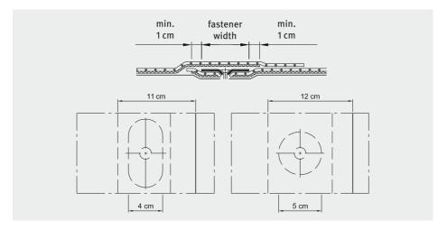
EVALON® waterproofing membranes are marked with several dashed lines along one longitudinal side. This **marking** can be used as a **guiding line** fort he corresponding lap width and is
