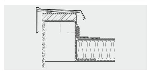
EVALON® VSKA tapes are produced with a non-coated approx. 12 cm wide welding edge on both sides (tape width 126 cm / 86 cm / 66 cm), or on one side (tape width 63 cm / 43 cm / 33 cm). Thus, a homogeneous welding of the EVALON® VSKA tapes to the roof sealing and the coated metal sheet angle is guaranteed.
