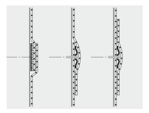
The spacing between the individual fasteners must not exceed 30 cm.
