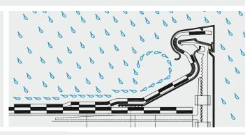
3 different varieties of top caps: 2,5 m long top caps in 3 different varieties for material-identical and tension-free flashing of the roof waterproofing; with mitred top cap sections for corners.
