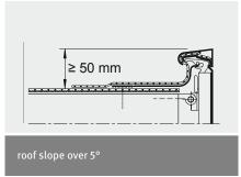
2 The roof edge trim profile must overlap the upper edge of the render finish or the façade cladding by at least 50 - 100 mm. The drip edge must have a minimum distance of 20 mm from the building structure. Relevant guidelines of the facade trades (plasterers) require drip edge distances of 40 mm for walls with thermal insulation composite systems (ETICS) and for plastered walls ≥ 40 mm. National regulations apply.
