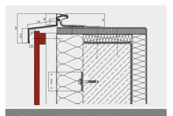
Installation over non-load bearing element (timber)
